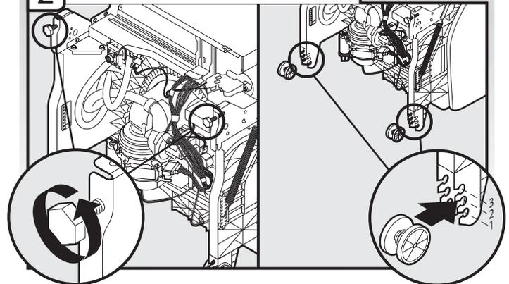
Turn both leveler legs to the same height. Put wheels in the required position determined from "Dishwasher Height Adjustment Chart." (To change wheel position, use a flat-blade screwdriver to pop out the wheel, then snap into the new position.)
